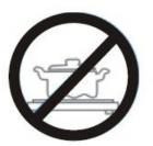
Do not place rough or uneven appliances, which may damage the ceramic surface.
