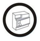
A dedicated power protection air switch must be incorporeted in the fixed wiring in accordance with the wiring rules.
