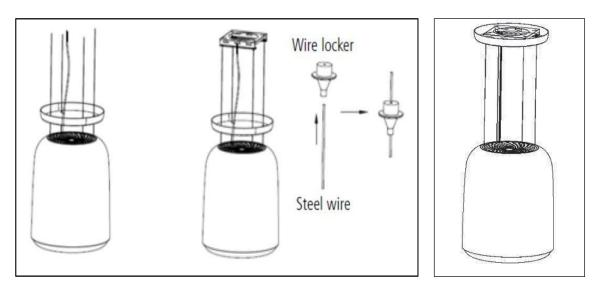
4) Push the fixing bracket cover up to the fixing bracket. Magnets will fix it in place.
