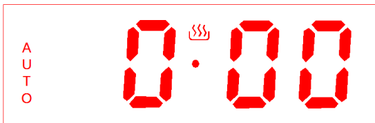
Pic 14 Cooking time setting initial state
